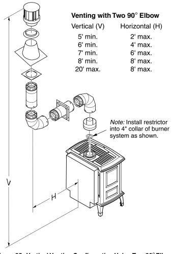
Figure 35 - Vertical Venting Configuration Using Two 90° Elbow
